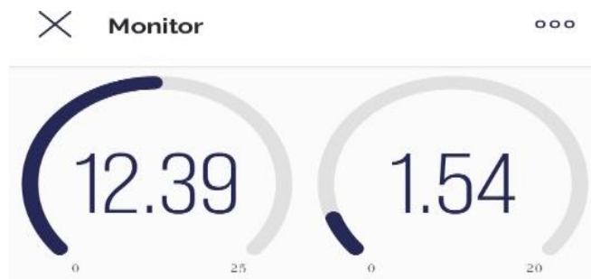
Figure 5: Reading of voltage and current for 1 day in gauge
