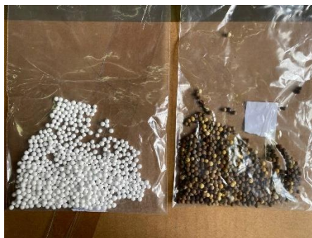
Figure 15: Different after 2 years the desiccant gel works in the air dryer
