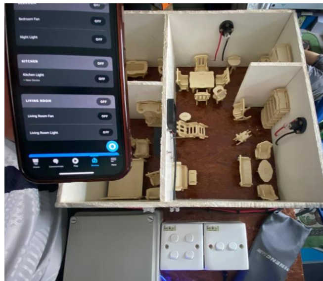
Figure 9: Example of step 0 from the truth table, both the manual switch and Alexa are set to off
