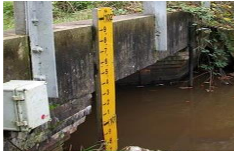
Figure 3: Current technology of water level indicator.
