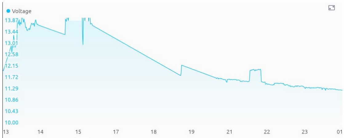
Figure 5: Voltage graph of 30W and 17Ah (Formula 2)
