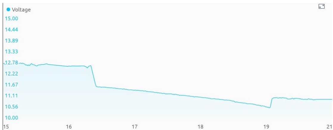
Figure 3: Voltage graph of 20W and 12Ah (Formula 1)
