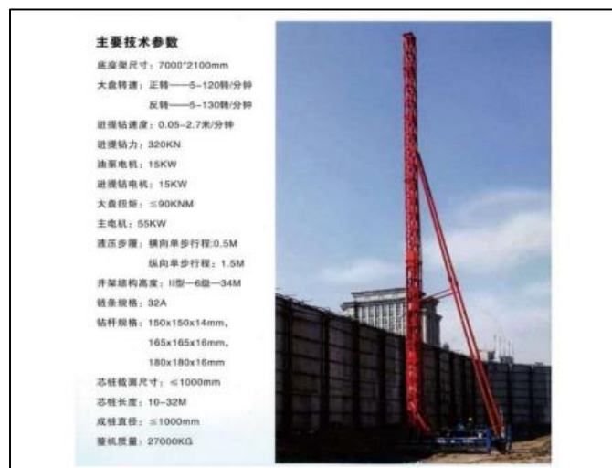
Figure 1: PH-5D Deep Soil Cement Mixing Pile Driver [8]
