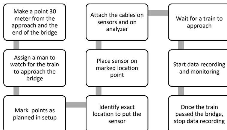
**Figure 1: Procedure of Vibration Test Plan**
