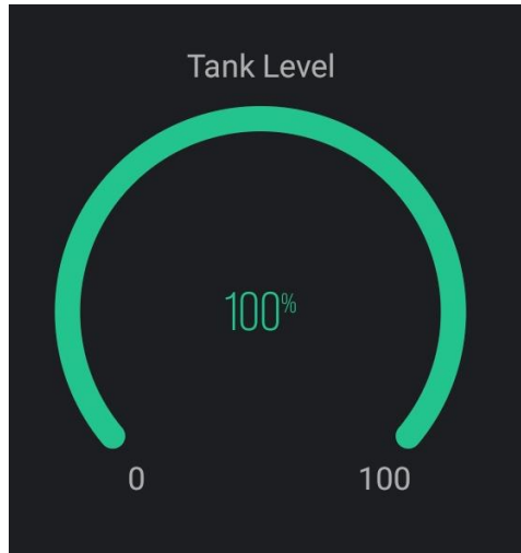
Figure 8: Blynk gauge display water level in main tank
