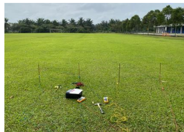
(b) Method used in soil resistivity
