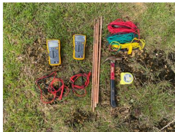
(a) Material used in soil resistivity
