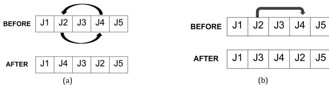
Fig. 1 (a) The method for swapping job locations in the flowshop scheduling; (b) The insert method between jobs
