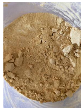
(c) Orange peels after blended and sieved through a 600 µm mesh size
