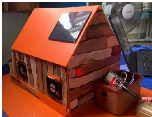
Figure 4: House's Replica Installed with Gas leakage Detection and Ventilation System
