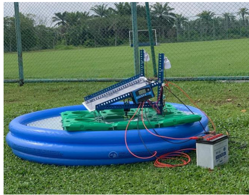
Fig 4 The prototype floating solar panel.
