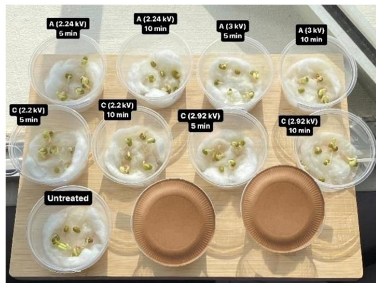
Fig 9 After 24 h of plasma treatment with copper (C) and aluminium (A) at different electrode configuration
