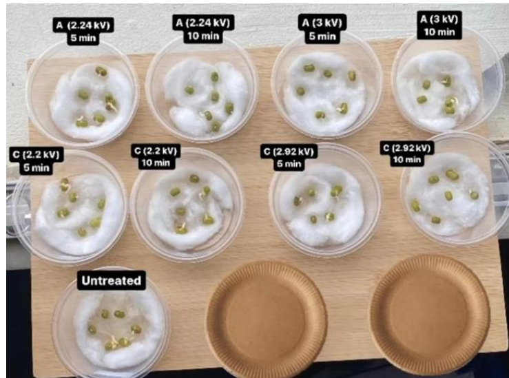
Fig 8 After 12 h of plasma treatment with copper (C) and aluminium (A) at different electrode configuration
