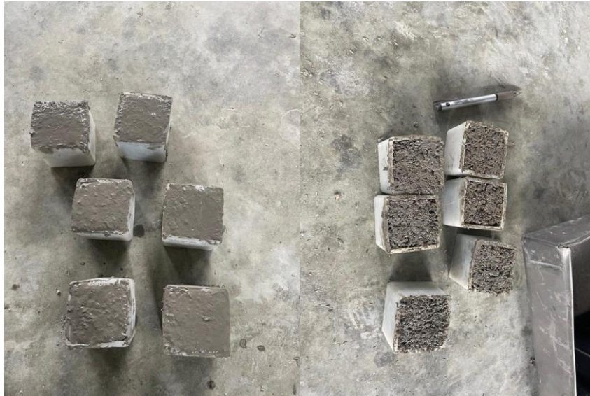
Figure 4: Moulded sample 50x50x50mm
