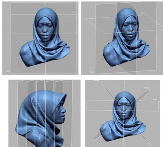
**Figure 2: Reference planes created for head scan alignment (HC-plane, BCA-plane and SA-plane)**
