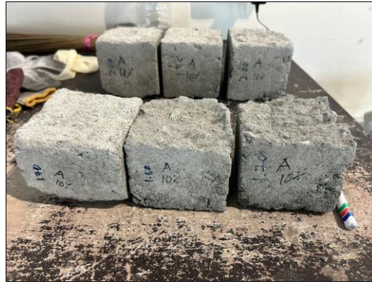
Fig. 8: The image of evidence of a crack on the test cube at 28 days on above 10% sand replacement with AD
