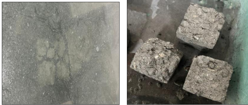
Fig. 10: Concrete cube crack during in process of curing tank causes imperfect size for sand replacement AD in 10%, 15%, and 20% at 28 days sample cube
