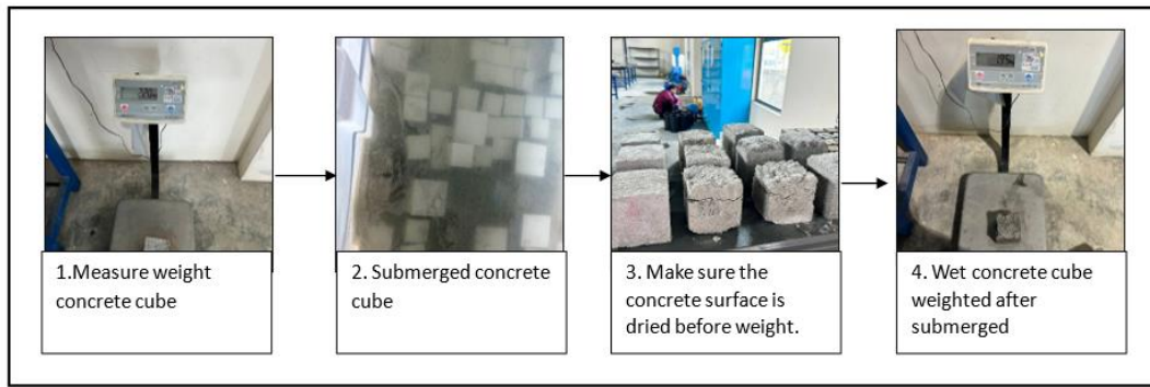
Fig. 4: Water absorption test procedure
