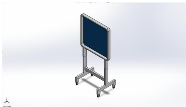
Fig. 2: Design A visualize a height adjustable foam type of visual display board
