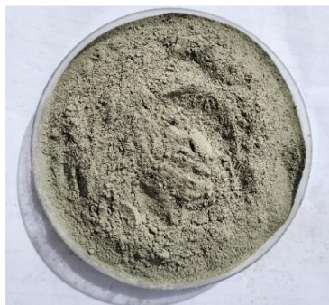
Fig. 5: Capillary crystalline waterproofing material
