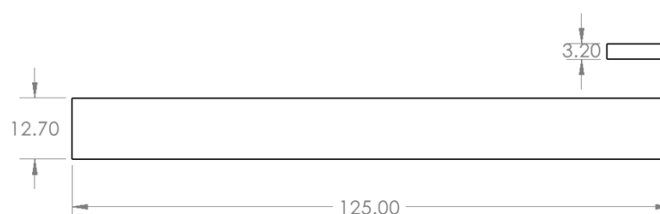
Fig. 5: ASTM D6110 standard dimension for rectangular with notch
