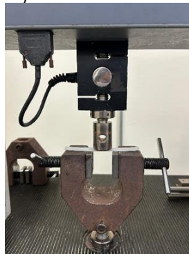
Fig. 10: The sample is being positioned in the universal testing machine
