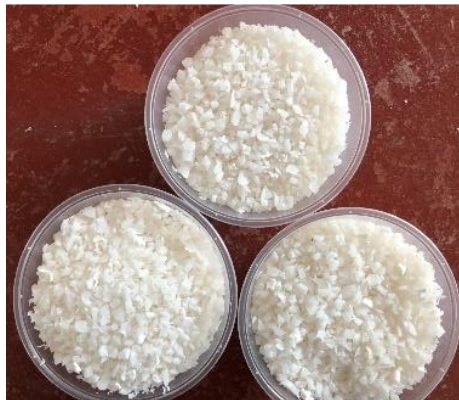
Fig. 1: 80% PP + 20% Crushed UHMWPE
