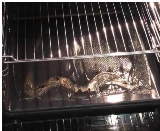
Fig. 4: shows the melted rubber powder after being put in the oven
