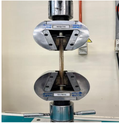
Fig. 7: The HPCs specimen being placed on the Universal Testing Machine for Tensile Strength Test
