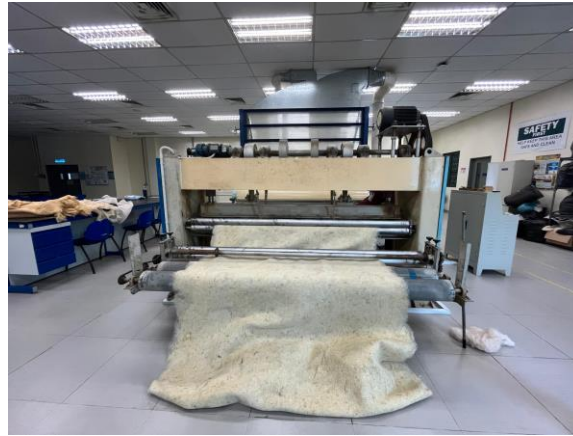
Fig. 2: Preparation of PALF-Polyester mat fiber
