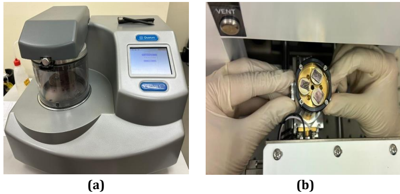
Fig. 3: SEM Testing (a) Coating with gold (AU) (b) Sample in COXEM machine
