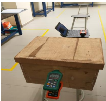
Fig. 7: Monotone sound and sound level meter for sound acoustic test
