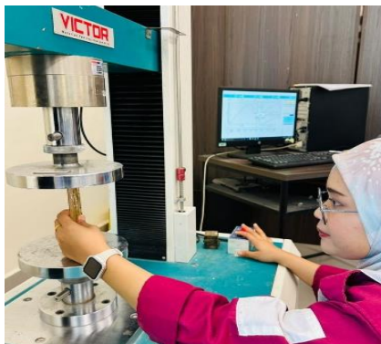
Fig. 6: Position the sample parallel to the surface between the plate during compressive test
