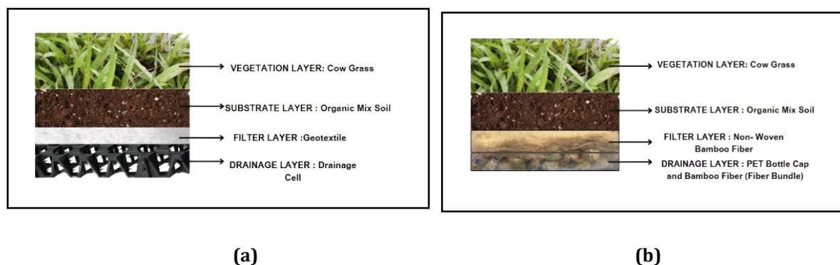
Fig. 1: Both model green roof in this study (a) conventional green roof (b) bamboo fibre green roof
