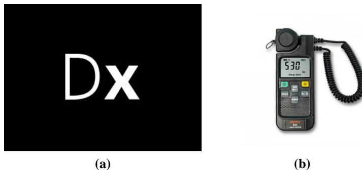
Fig. 1: Software and tools (a) Dialux software; (b) Lux meter
