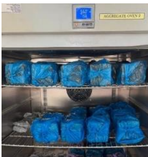
Fig. 4: The sample of geopolymer concrete covered with plastic to complete the curing in oven.
