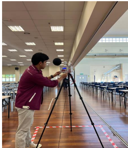
Fig. 2: On- site measurement using thermal comfort kit (LSI Lastem heatshield)
