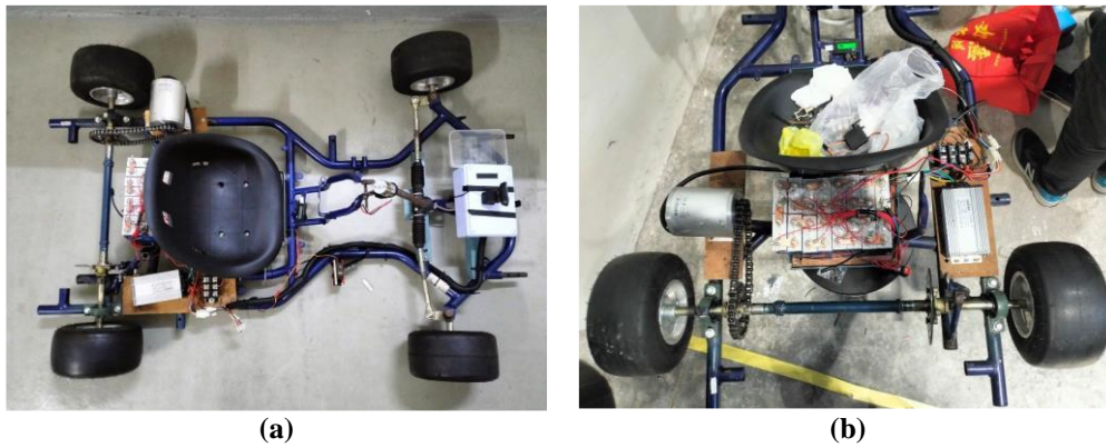
Fig. 2: Experiment Setup (a) Top view of full Go-Kart (b) Back view of Go-Kart for Acceleration part
