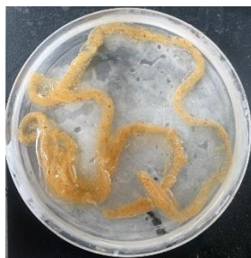
Fig. 9: Sample A extruded in acetone bath
