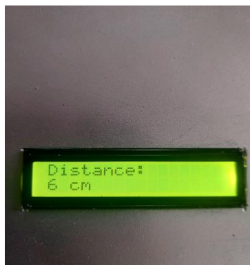
Fig. 7: Example of real-time data displayed on the LCD
