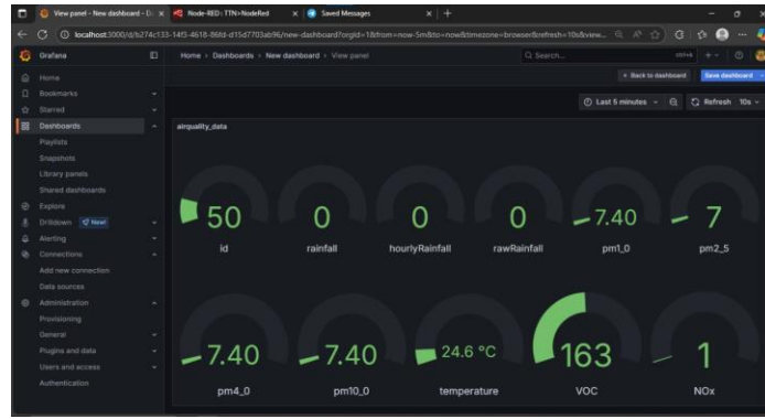
Fig. 5 Grafana Dashboard Showing PM, VOC, Temperature, and Humidity Readings
