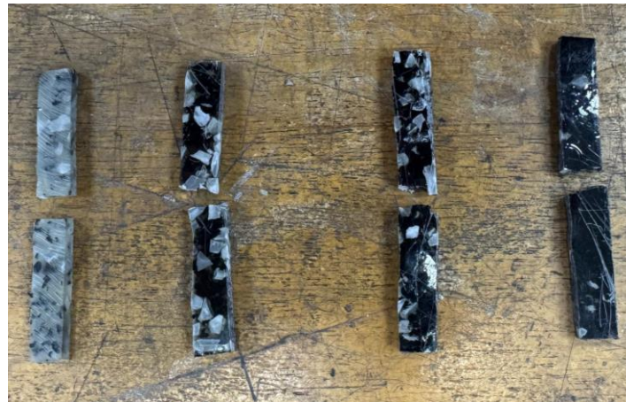
Fig. 9: Sample After the Impact Test
