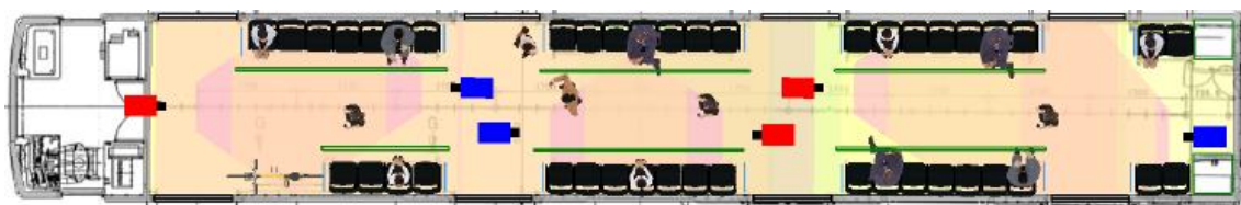
Figure 9 – Optimized Camera Placement for Cab Coach
