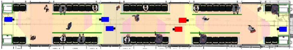
Figure 10 – Optimized Camera Placement for Middle Coach
