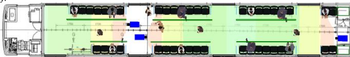
Figure 7 - Existing Camera Placement for Cab Coach
