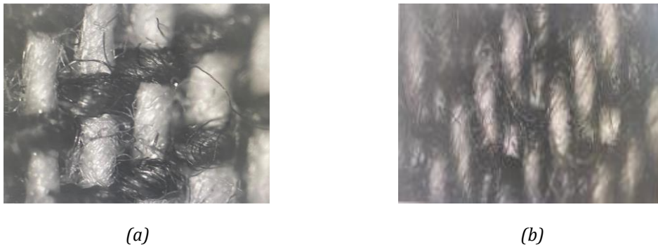
Fig. 4 Surface morphology Denim 3 (a) Uncoated (b) Coated
