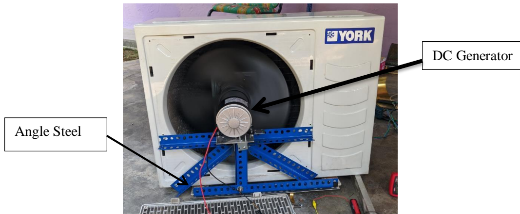
Figure 3: Angle Steel used to hold the Generator
