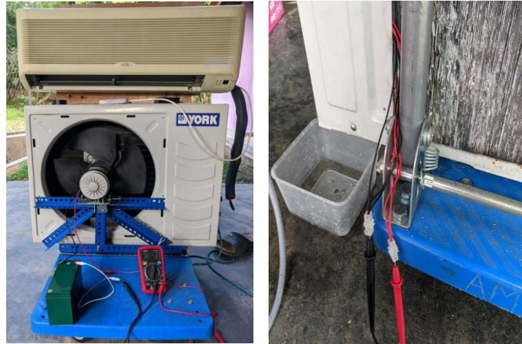
Figure 5: Prototype of a 1 HP air-conditioner a) The Front Design of Compressor b) Behind the Compressor
