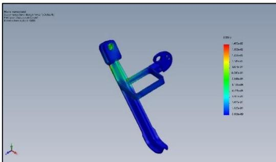
Figure 19: Strain of side stand
