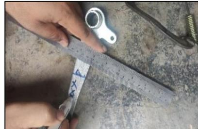
**Figure 9: Marking process**
