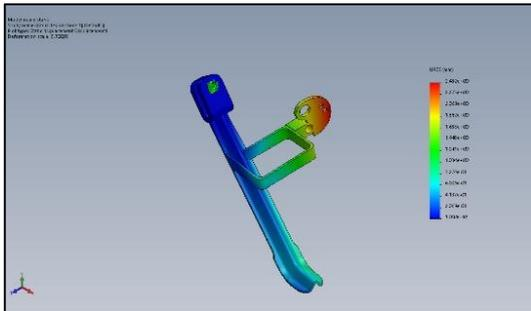
Figure 17: Displacement of side stand
