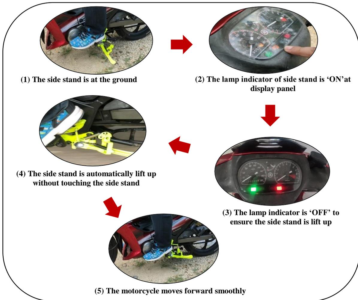
**Figure 24: Functional test result**
