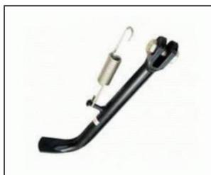
**Figure 1: Manual side stand of Yamaha 125ZR**
