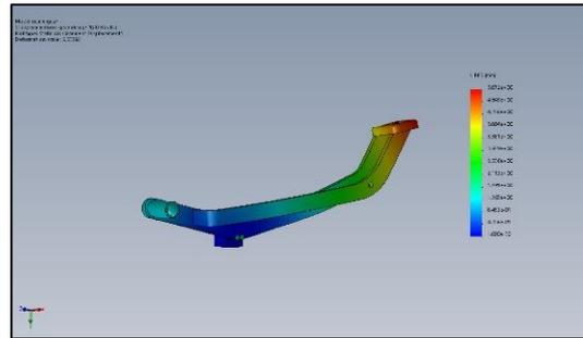
Figure 18: Displacement of gear lever
