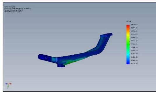
Figure 20: Strain of gear lever
