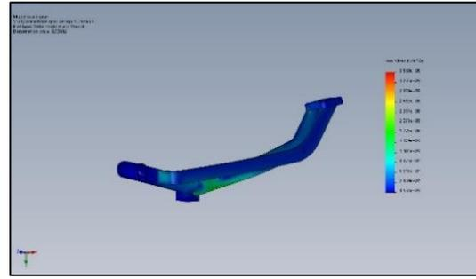
Figure 16: Stress of gear lever
