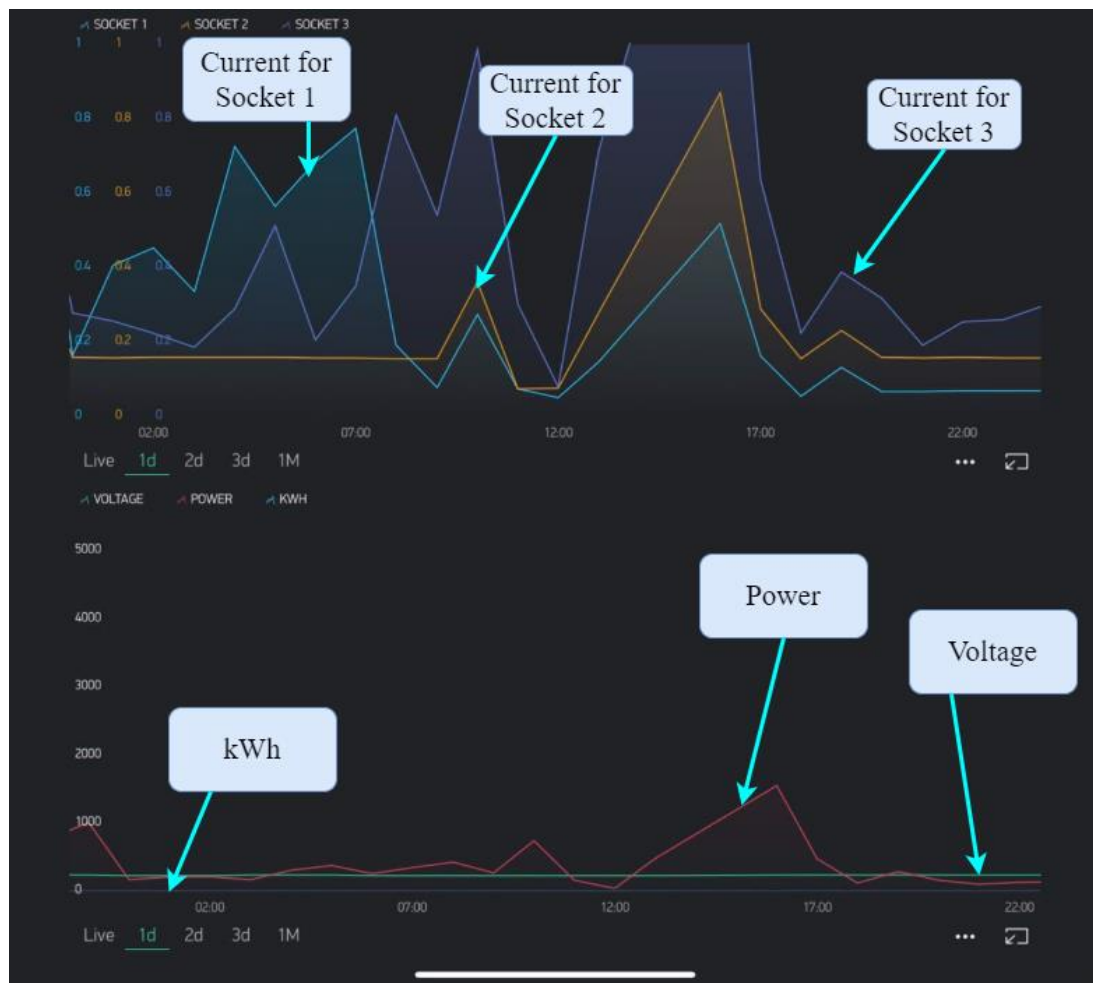
Figure 10: Power usage for 1 day of Smart DB monitoring
