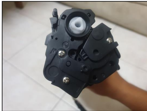
Figure 12: Secondary body left cover screws location
