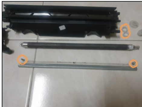
Figure 7: Eliminated cleaning blade screws and developer roller cover
