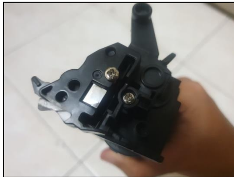
Figure 11: Main body left cover screws location
