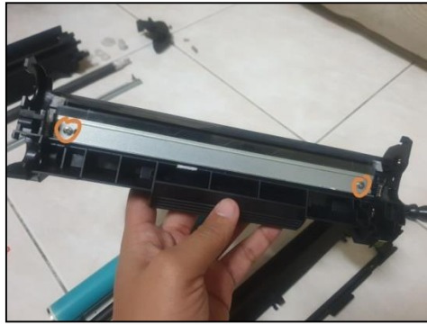
Figure 9: Eliminated cleaning blade screws
