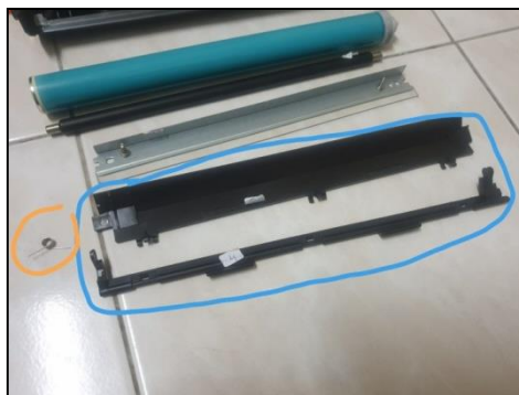
Figure 8: Eliminated locking spring and combined OPC drum cover
