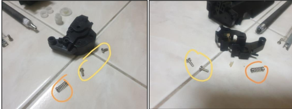
Figure 6: Eliminated spring and reduced screws
