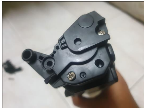
Figure 10: Main body right cover screws location
