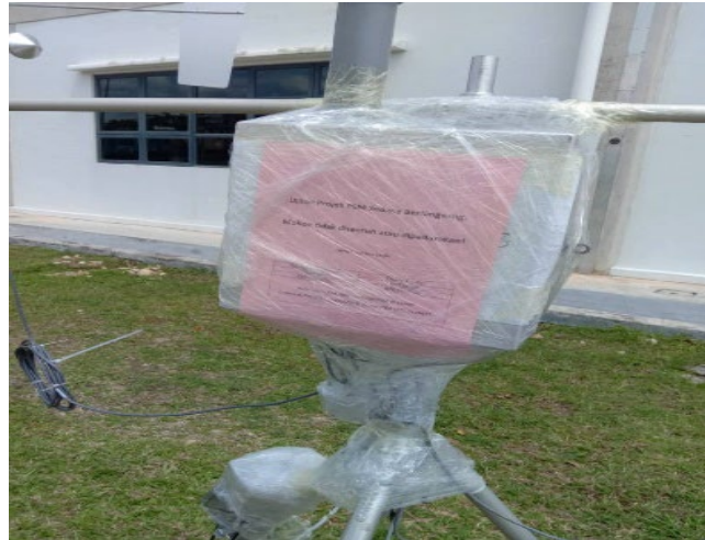
Figure 4 (b): Wrapped the E-sampler to water-resistant
