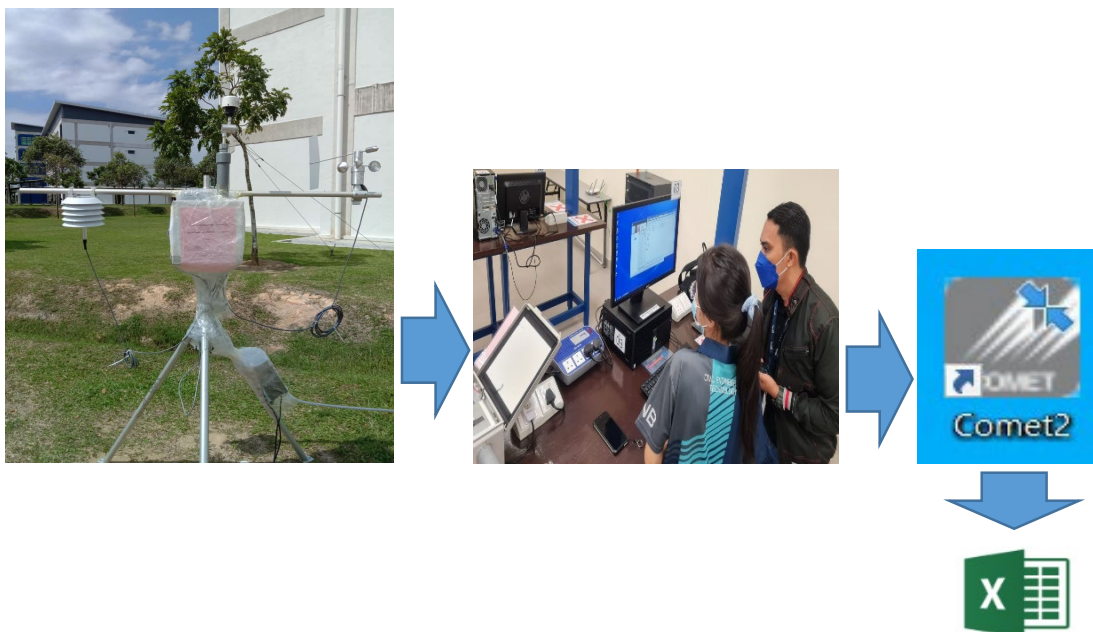
Figure 12: Operation of an E-sampler dual ambient monitor with the conventional framework
