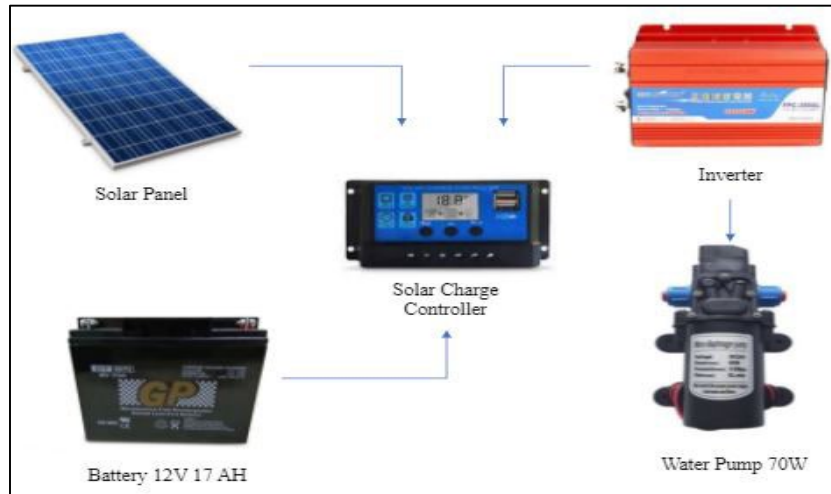
Figure 2: Block diagram of Lake Bin Machine
