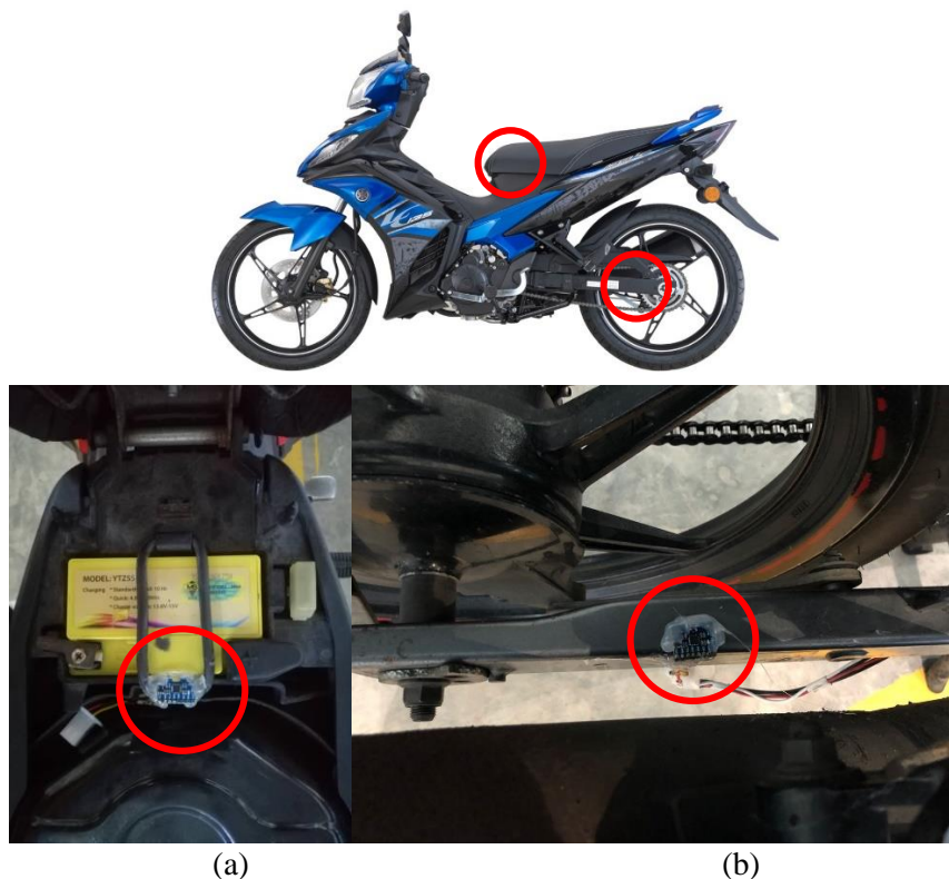
Figure 3: Position of the gyro sensor at (a) sprung (b) unsprung
