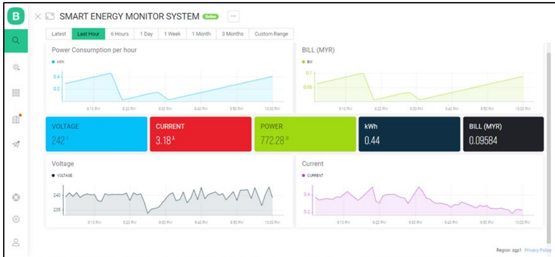
Figure 7: Sensors and power consumption reading in Blynk website
