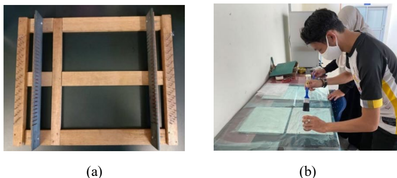
Figure 2: (a) Weaving loom and (b) Hand lay-up process
