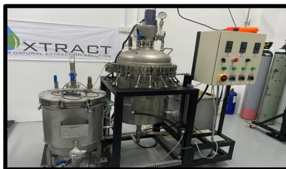
Figure 1: The 70-L sub-critical water extractor
