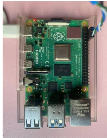
Figure 6: Raspberry Pi GPIO Port Connection
