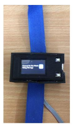
Figure 5: Prototype of Smartwatch
