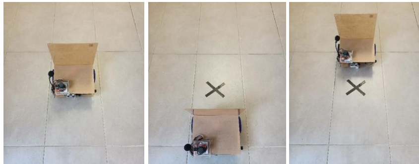
Figure 10: Wheelchair prototype moves forward and backward from initial position
