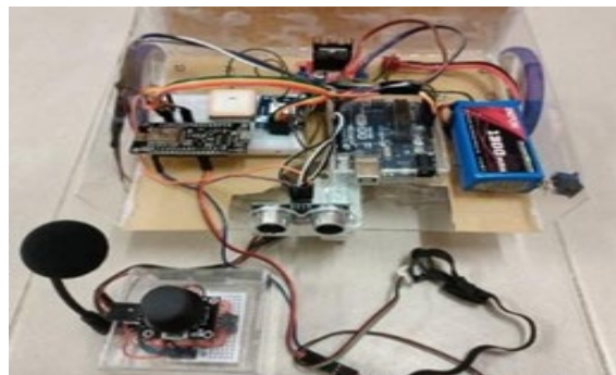
Figure 7: Circuit connection of the wheelchair prototype
