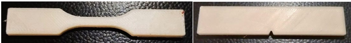
Figure 3: Tensile sample (ASTM D638 Type V) and Izod impact sample (ASTM D256)
