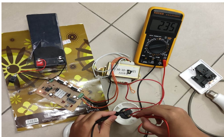
Figure 15: Measure the output inverter
